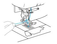
**5** Pull out about 10 cm (4 inches) of the bobbin thread under the presser foot toward the rear of the machine.
